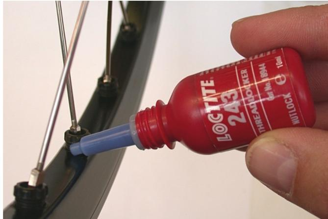
Then tighten the cups in place. Mavic say use a torque of 5.5Nm, I'm not sure what that feels like but using the Mavic wrench I give it a firm twist (bit ambiguous), watch out if using the Park wrench because there's more leverage on that one and a danger of over tightening.
